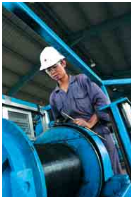
Wireline spooling on a reel skid.
